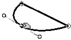
Selecting a control point on a curve
